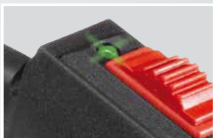
The multi-coloured LED shows the current arc trim condition selected.
