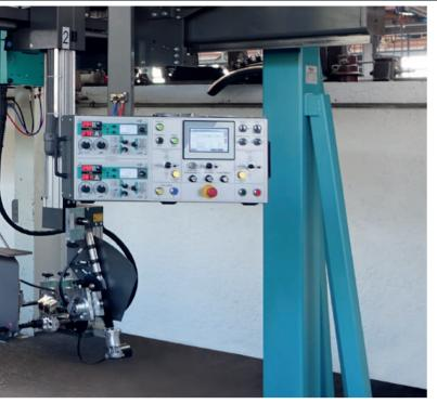
With the Merkle longitudinal welding machine, longitudinal beams may be welded simultaneously and automatically to any length. The construction permits a high economical solution for MIG/MAG and PulseARC welding in different geometrics of fillet and butt weld preparation.
