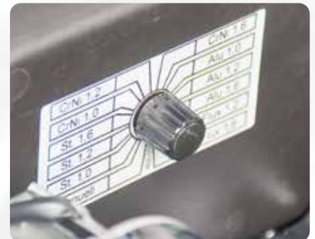
Material and wire diameter selection inside the wire feeder.
