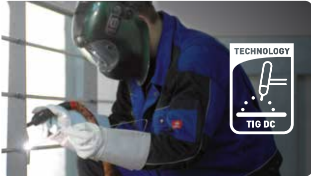
1. Steel / stainless steel welding in DC
