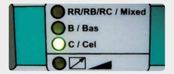
Choose between three kinds of electrode types through the new designed and clearly arranged operating panel. Different characteristic curves for several electrode types:
